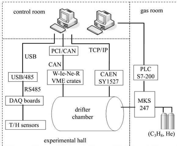
Fig. 1. Schematic diagram of the system hardware architecture.
