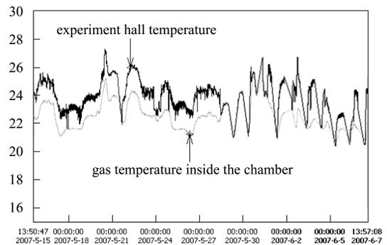
Fig. 5. Temperature of the chamber inside and the experimental hall.
