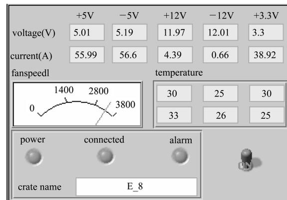
Fig. 2. Graphical user interface for a single VME crate monitoring and control.
