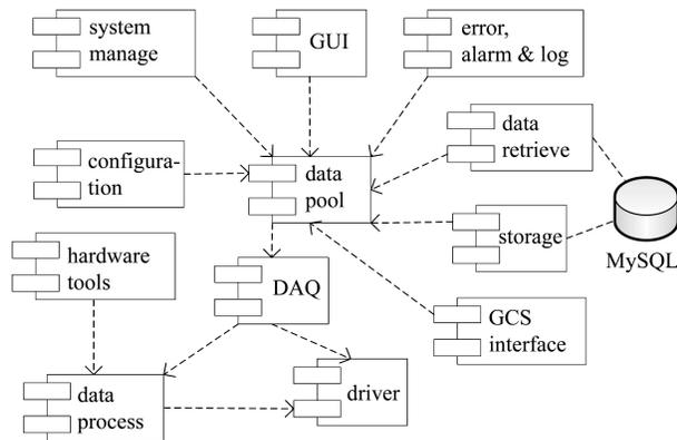
Fig. 4. Architecture of the top level supervisory and control software.
