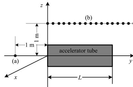
Fig. 3. Coordinate to calculate the radiation distribution of lost electrons.
