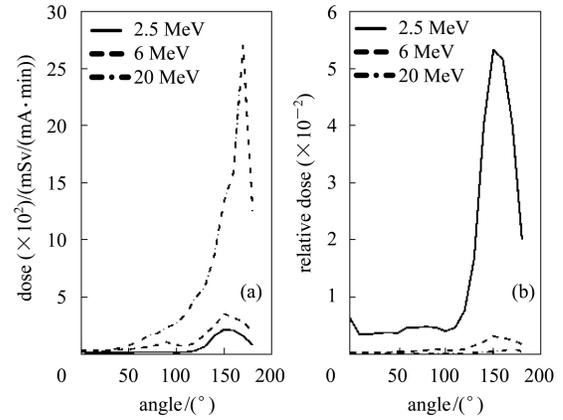
Fig. 5. Leaking dose distribution of lost electrons in the three accelerators.
