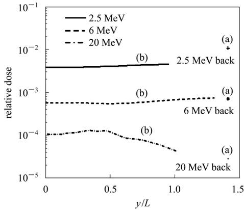
Fig. 4. Leaking dose rate along the axis of the three accelerators.
