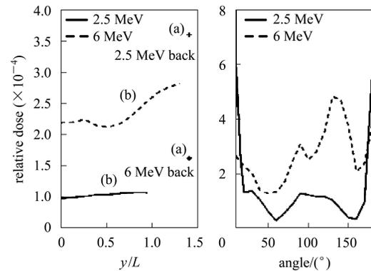
Fig. 6. Shielded leaking dose rate distribution in 2.5 and 6 MeV accelerators.
