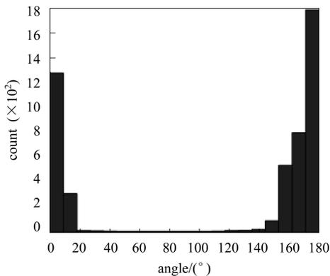
Fig. 2. Diverging angular distribution of lost electrons in 6 MeV accelerator.
