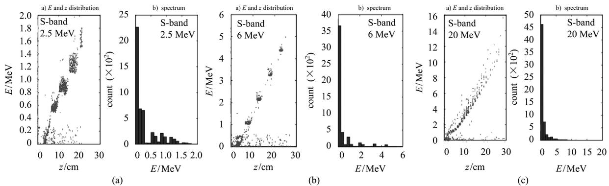
Fig. 1. Spectrum-location distributions of lost electrons in S-band SW accelerator of energies of (a) 2.5 MeV, (b) 6 MeV and (c) 20 MeV.
