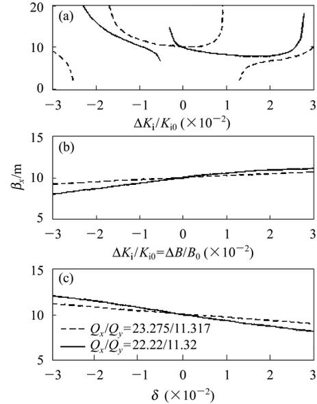
Fig. 5. The  $\beta$  function beating in the center of the long straight section of two working.
