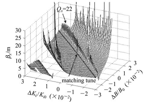
Fig. 4. Variation of the horizontal  $\beta$  function in the center of long straight section generated by field errors with all the sextupoles on in the SSRF storage ring.
