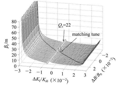
Fig. 2. Variation of the horizontal  $\beta$  function in the center of long straight section generated by field errors with all the sextupoles off in the SSRF storage ring.
