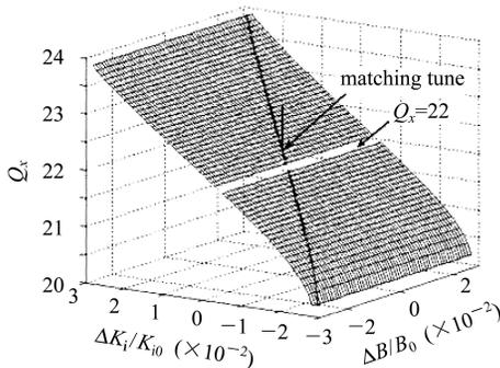
Fig. 1. Variation of the horizontal working point generated by field errors with all the sextupoles off in the SSRF storage ring.
