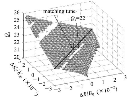
Fig. 3. Variation of the horizontal working point generated by field errors with all the sextupoles on in the SSRF storage ring.
