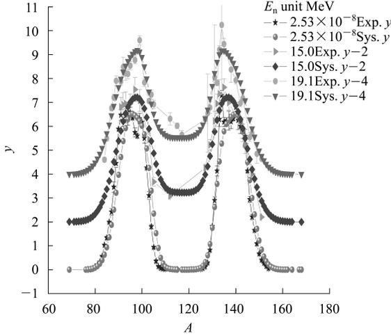
Fig. 5. The comparison of the yield calculated by systematics with the data measured by RAM method.
