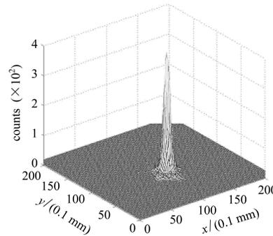
Fig. 6. Point Spread Function of 140 keV gamma rays. A spatial resolution of 3.1 mm FWHM is obtained.
