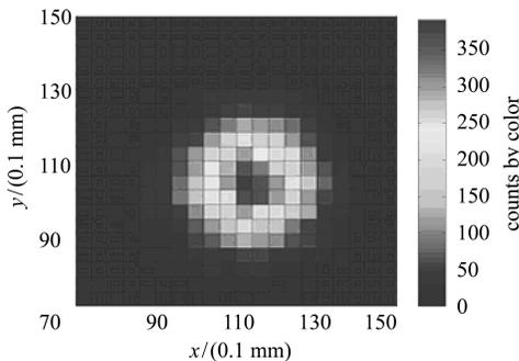
Fig. 5. Image of 140 keV gamma rays.
