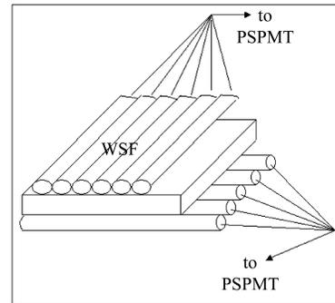
Fig. 1. A schematic diagram of the simulation prototype.
