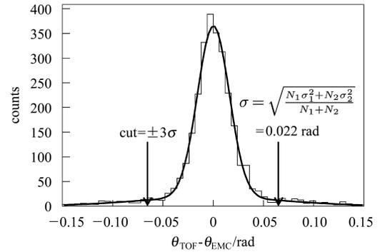
Fig. 7. TOF and EMC match in  $\theta$  direction. The histogram is fitted with a double-Gaussian and the matching window is  $|\Delta\theta| < 3\sigma$ .  $N_i$  and  $\sigma_i$  ( $i=1,2$ ) denote the area and standard deviation of  $i$ th Gaussian, respectively.
