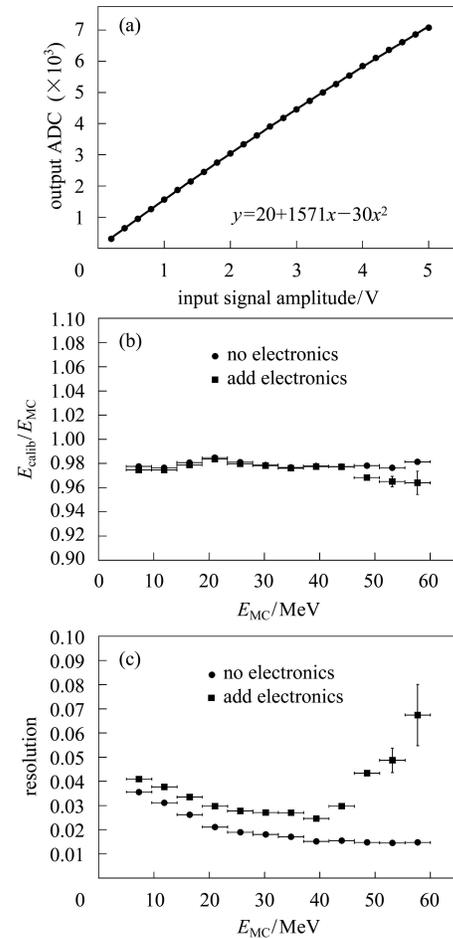
Fig. 5. (a) Linearity of the TOF readout electronics. The points are the measured data, and the curve is the fitted function. (b) Energy linearity. (c) Energy resolution as a function of energy deposit.
