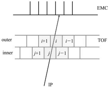
Fig. 6. TOF and EMC match in  $\phi$  direction.
