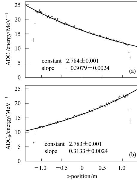
Fig. 4. Charge collected as a function of the hit position, (a) the west end and (b) the east end. The fitted functions are exponentials.
