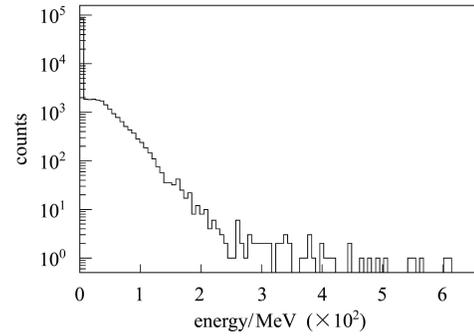
Fig. 2. Energy deposit in TOF for 1 GeV photons.
