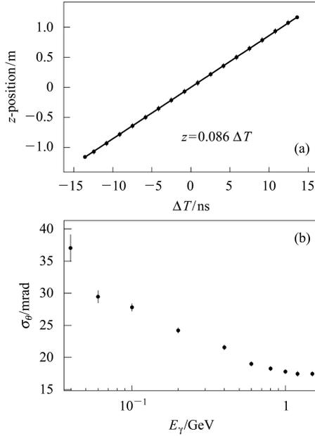
Fig. 3. (a) Hit position as a function of timing difference between the two ends of the scintillator, together with the fitted function. (b) The  $\theta$  resolution as a function of the incident photon energy.
