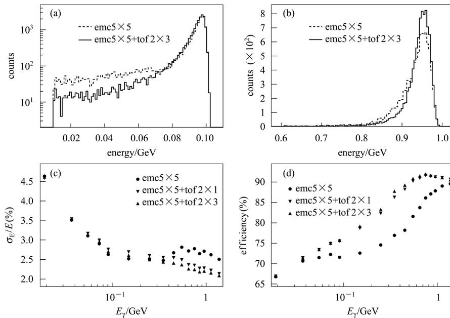
Fig. 8. Reconstructed energy distribution in EMC for (a) 0.1 GeV and (b) 1 GeV photons. The broken line is for EMC only, while the solid line with TOF correction. (c) and (d) the distribution of energy resolution and detection efficiency as a function of incident photon energy, respectively.
