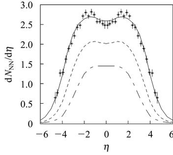
Fig. 3. Pseudorapidity distribution in p+p collisions at  $\sqrt{s}=200$  GeV. The stars are the results from the UA5 collaboration. The solid line is the result from Eq. (10). The dashed and dash-dotted lines are the results for p+p collisions at  $\sqrt{s}=62.8$  GeV and  $\sqrt{s}=20$  GeV, respectively.
