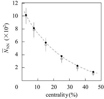
Fig. 2. The centrality dependence of the mean number of binary nucleon-nucleon collisions in Au+Au collisions at  $\sqrt{s_{NN}} = 200$  GeV. The solid circles are the results from Eq. (8), the open circles the results given by the BRAHMS collaboration.
