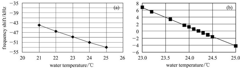
Fig. 6. Frequency shift versus water-cooling temperature. (a) Stainless-steel; (b) Copper.
