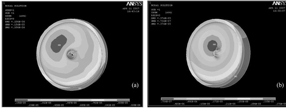
Fig. 4. Structural distortion for (a) Stainless-steel; (b) Copper.
