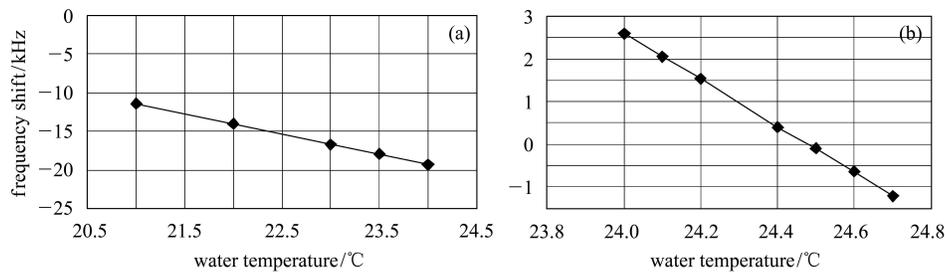
Fig. 7. Frequency shift versus water-cooling temperature with nose-cone cooling. (a) Stainless-steel; (b) Copper.
