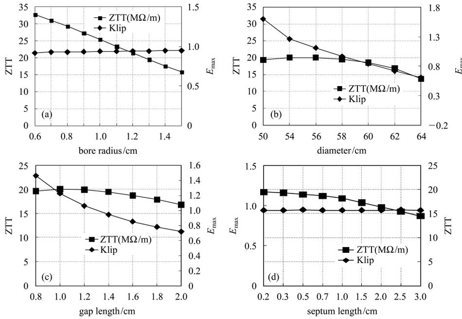
Fig. 2. (a) Bore radius (cm) versus shunt impedance ( $M\Omega/m$ ) and Kilpatrick limit; (b) Diameter (cm) versus shunt impedance ( $M\Omega/m$ ) and Kilpatrick limit; (c) Gap length (cm) versus shunt impedance ( $M\Omega/m$ ) and Kilpatrick limit; (d) Septum length (cm) versus shunt impedance ( $M\Omega/m$ ) and Kilpatrick limit.
