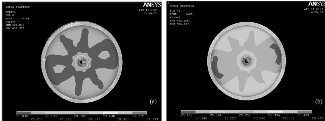
Fig. 3. Temperature distribution with water-cooling, (a) Stainless-steel; (b) Copper.
