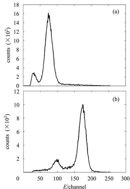
Fig. 3. The typical energy response of two detectors: (a) CCD and (b) ACD.
