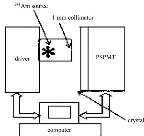
Fig. 1. The block diagram of the measure instrument.
