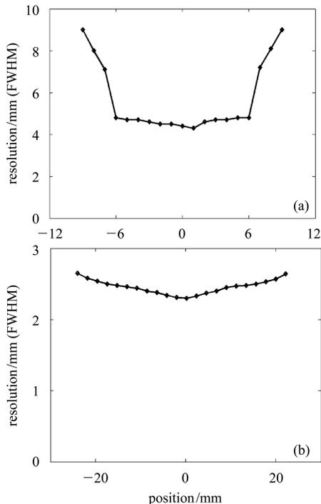
Fig. 6. Spatial resolution response as a function of position: (a) CCD and (b) ACD.
