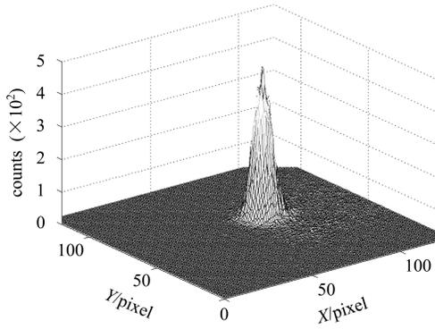
Fig. 4. A typical point spread function (PSF) of CCD.
