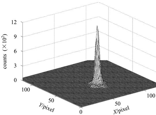
Fig. 5. A typical point spread function (PSF) of the ACD.
