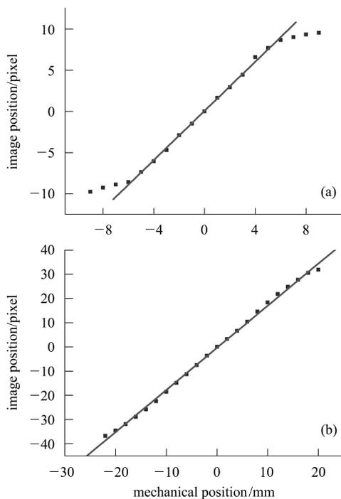
Fig. 2. The position linearity response of two detectors: (a) CCD and (b) ACD.
