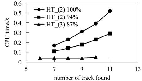
Fig. 4. Correlation of time-consuming of CPU and track number by using different type of Hough Transform method.
