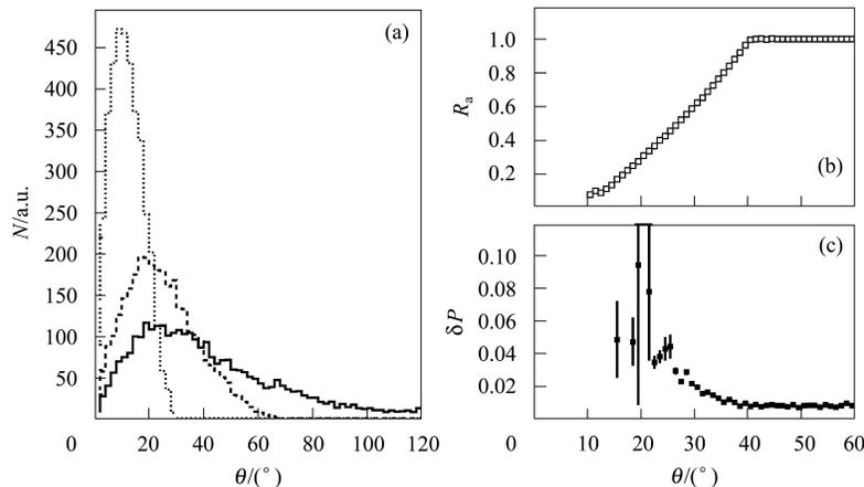
Fig. 1. (a) Angular distribution for products K(dotted), p(dashed),  $\pi$ (solid) of reactions  $pp \rightarrow p+p+\phi (\rightarrow K^+ K^-)$  and  $pp \rightarrow p+n+\pi^+$ ; (b) Effective thickness  $R_a$  in laboratory; (c) Single track momentum resolution of TPC versus the polar angle in laboratory.
