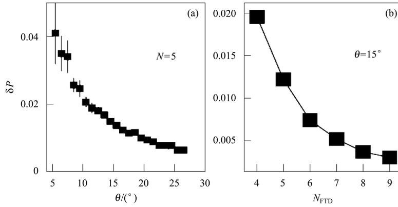
Fig. 2. (a) Single particle momentum resolution versus angle of FTD in laboratory; (b) Correlation of single particle momentum resolution and number of MWDCs being used at polar angle  $15^\circ$  in laboratory.
