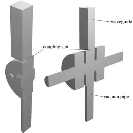
Fig. 4. 3-D MAFIA model for the coupler design of 1-cell (Left) and 3-cell (Right) structure.
