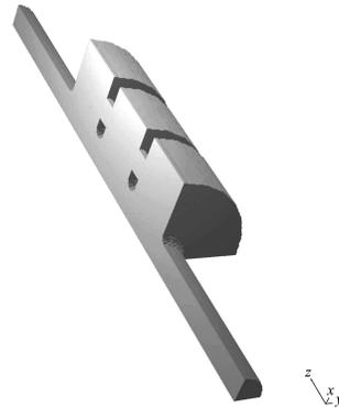
Fig. 2. 3-D MAFIA model of the 3-cell deflecting cavity with polarization holes.
