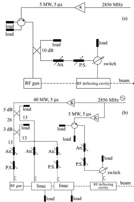
Fig. 6. (a) Power feeding system from 5 MW klystron with beam energy 3.5 MeV. (b) Power feeding system from 45 MW klystron with beam energy 50 MeV.
