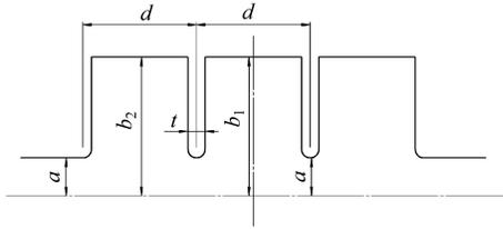
Fig. 1. 2-D geometry of the 3-cell deflecting cavity.
