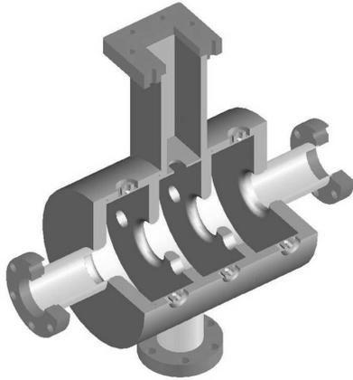
Fig. 5. CAD model for the 3-cell deflecting cavity.
