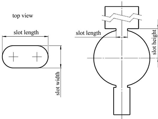
Fig. 3. Shape and dimension of the coupling slot.
