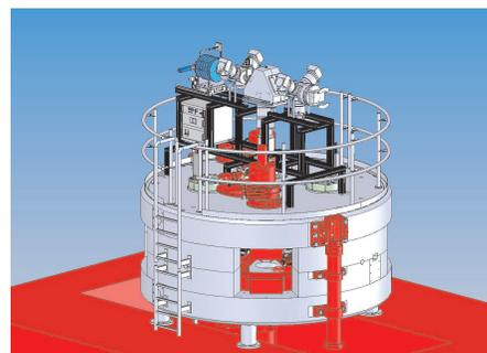
Fig. 7. Full injection bench mounted on the top of the C70 IBA cyclotron yoke.
