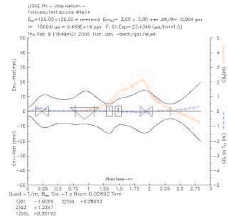
Fig. 5. Calculated envelope of the  $\text{H}^-$  beam.
