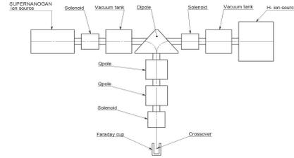
Fig. 3. Schematic view of the injection beam in the C70 IBA cyclotron.
