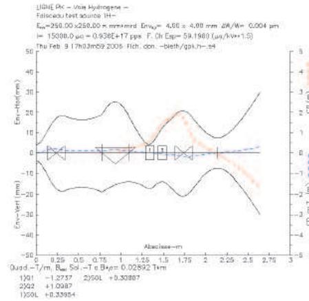
Fig. 4. Calculated envelope of the  $\text{He}^{2+}$  beam.
