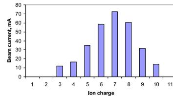
Fig. 4. Platinum ion charge state distribution at the optimal conditions.
