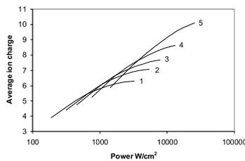
Fig. 3. Calculations of average ion charge of platinum in the plasma. Vacuum arc current: 1 – 100A, 2 – 150A, 3 – 200A, 4 – 300A, 5 – 500A.
