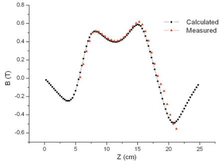
Fig. 2. The measured and calculated axial magnetic field.
