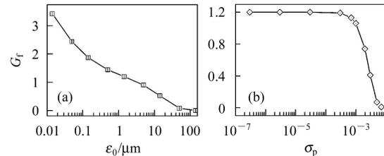
Fig. 5. The dependence of  $G_f$  on (a)  $\varepsilon_0$  with  $\sigma_p=3 \times 10^{-5}$ ; (b)  $\sigma_p$  with  $\varepsilon_0=1\mu\text{m}$ , other parameters:  $\gamma=60$ ,  $B_w=0.9T$ ,  $\lambda_w=3\text{cm}$ ,  $N=20$ ,  $\lambda=20\mu\text{m}$ .
