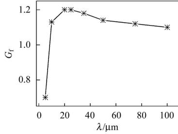
Fig. 2. The dependence of  $G_f$  on  $\lambda$ , parameters:  $\gamma=60$ ,  $B_w=0.9T$ ,  $\lambda_w=3\text{cm}$ ,  $N=20$ ,  $\varepsilon_0=1\mu\text{m}$ ,  $\sigma_p=3 \times 10^{-5}$ .
