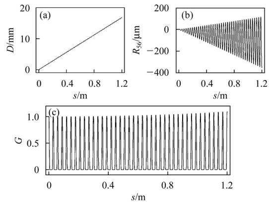
Fig. 1. (a)  $D(s)$ ; (b)  $R_{56}(s)$ ; (c)  $G(s)$  for the BFEL wiggler, parameters:  $\gamma = 60$ ,  $B_w = 0.3\text{T}$ ,  $\lambda_w = 3\text{cm}$ ,  $N = 40$ ,  $\lambda = 20\mu\text{m}$ ,  $\varepsilon_0 = 1\mu\text{m}$ ,  $\sigma_p = 3 \times 10^{-5}$ .
