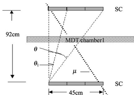
Fig. 2. The trigger system for cosmic-ray test.
