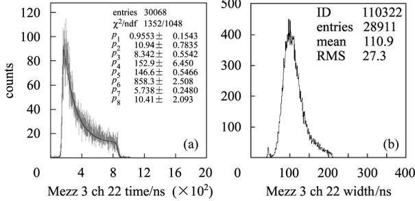
Fig. 4. (a) The drift time spectrum of one channel; (b) The charge distribution of the same channel.
