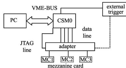
Fig. 3. The read-out electronics for the MDT chamber.
