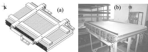
Fig. 1. (a) Schematic drawing; (b) Picture of BEE chamber with gas manifolds.
