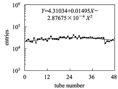
Fig. 6. The tube occupancy mapping in one tube row.
